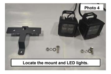
5. Install the lights facing forward onto the light mount using the supplied hardware included with the LED light kit. The longer tab will be toward the front of the vehicle when installed. Snug the hardware installed using a 14mm wrench See Photos 5 and 6.
