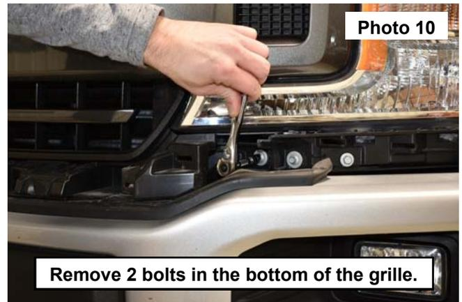
10. Remove the grille from the vehicle, set in a safe place to install the lights. **See Photo 11.**
