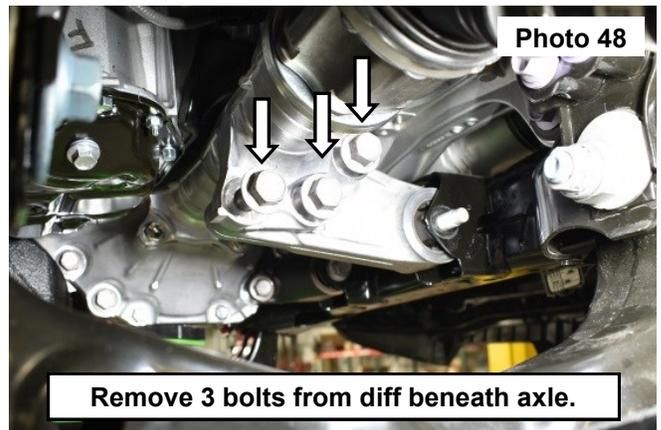
48. Remove the stock diff bracket beneath the axle. **See Photo 49.**
