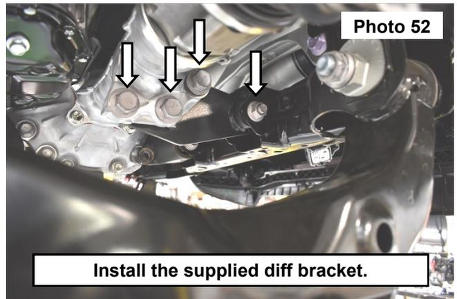
52. Install the diff bracket spacer and diff bracket beneath the diff using stock hardware at the frame and supplied 14mm x 65mm bolts and (2) 14mm flat washers in the diff using a 22mm socket/wrench. **See Photo 53 and Photo 54.**
