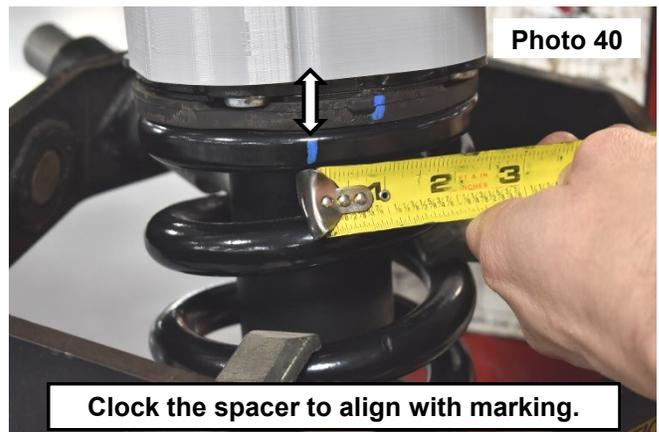
40. Install the strut into the vehicle with the supplied 10mm flange nuts using a 15mm wrench and install the new upper control arm using the stock hardware. **See Photo 41.**
