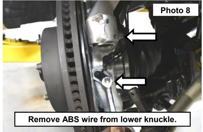
10. Remove the ABS wire and brake line bracket from the knuckle using a 10mm & 12mm socket/wrench. **See Photo 9.**
