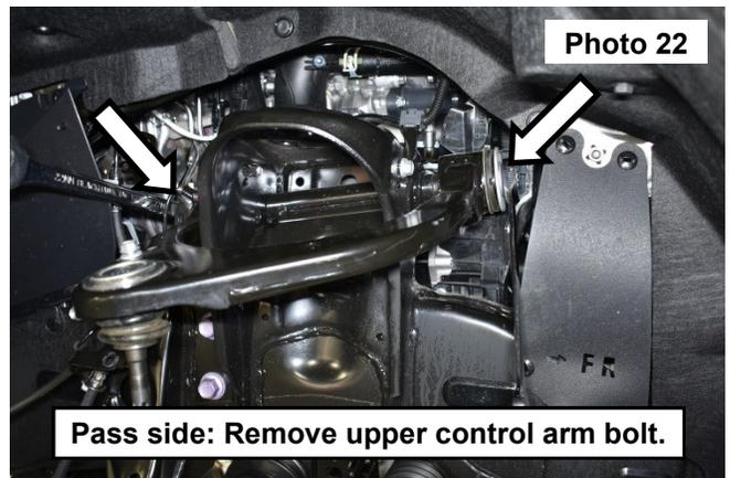
22. Slide the bolt out to remove the upper control arm. **See Photo 23.**
