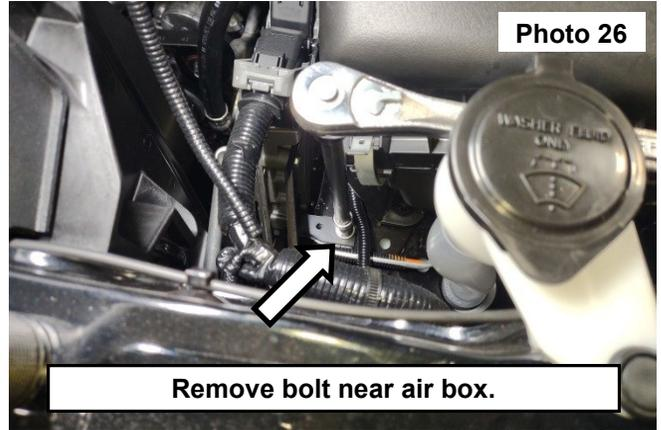
26. Remove the bolt near the washer fluid refill using a 10mm wrench. **See Photo 27.**
