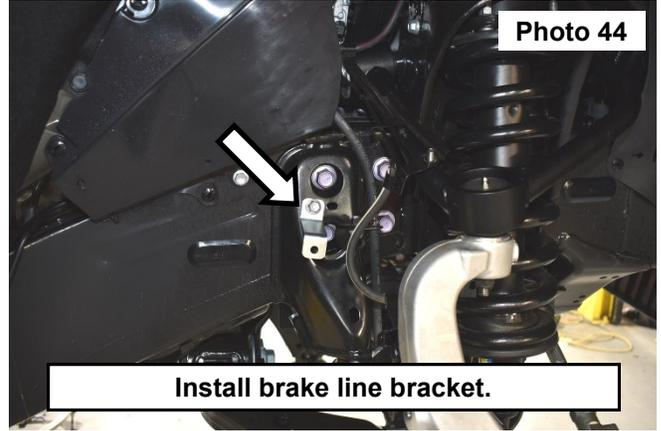
44. Install the brake line to the brake line bracket using the supplied 5/16" x 3/4" bolts, washer, and flange nut. Tighten using two 13mm socket/wrenches. **See Photo 45.**
