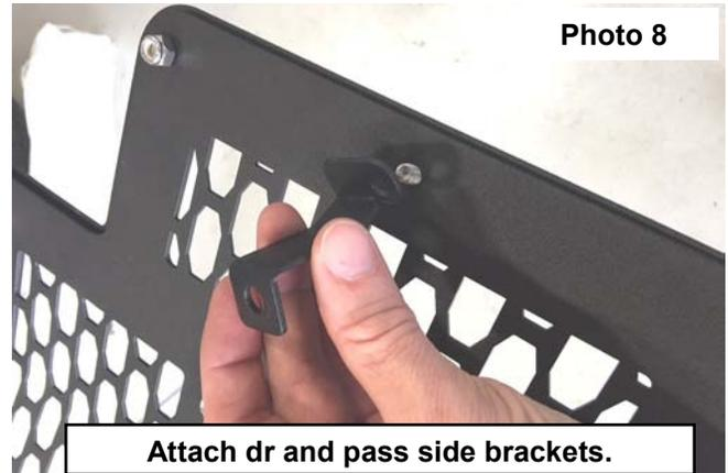
10. Attach the driver and passenger brackets to each side of the grille using the supplied 1/4" x 5/8" bolts and nuts. Tighten using a 5/32" Allen and 7/16" wrench. **See Photos 8 & 9.**
