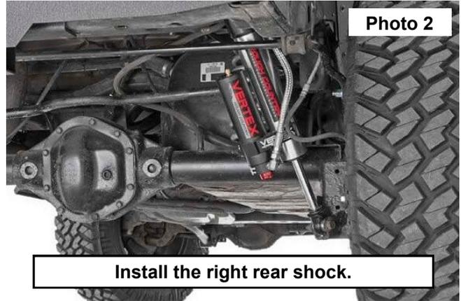
2. Torque the factory hardware in the top of the shock to 35 ft-lbs. using a 16mm socket.
