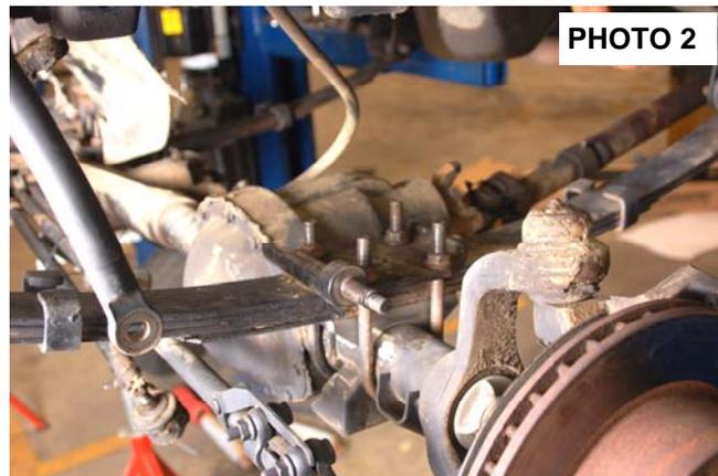
7. Reinstall the axle under the springs and double check the pinion angle and spring width. When properly positioned, weld spring pads onto the axles. Take care not to use excessive heat when welding the spring perches on the axles.
