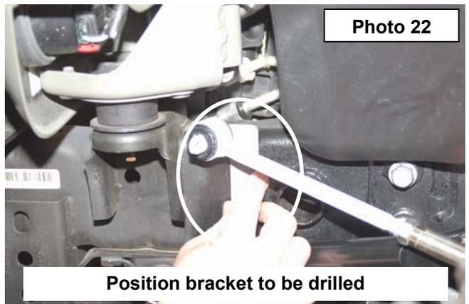
**Position bracket to be drilled**
