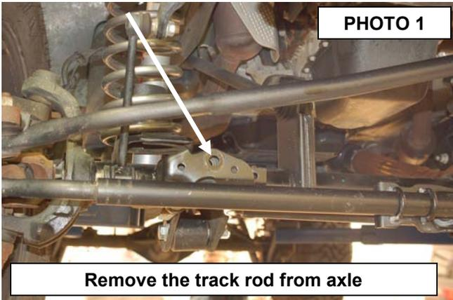
Remove the track rod from axle
