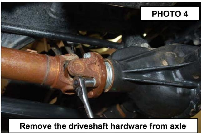
Remove the driveshaft hardware from axle
