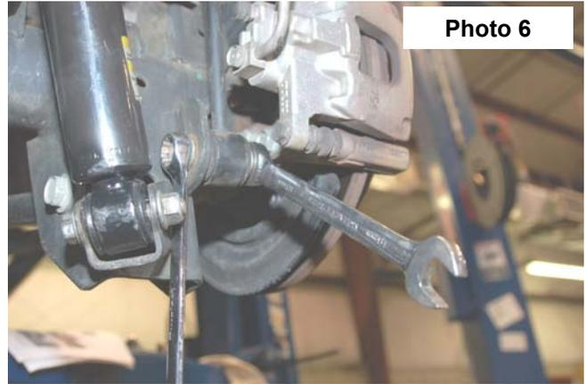
5. Using a 10mm wrench remove the bolt holding the brake line to the frame. **See Photo 7.** Push down on the axle to allow enough room for stock coil spring to be removed. Remove the stock coil spring and isolator.
