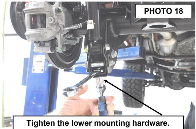
20. Tighten the lower shock bracket bolt using a 3/4" socket and wrench. Torque to 65ft/lbs. **See Photo 18.**
