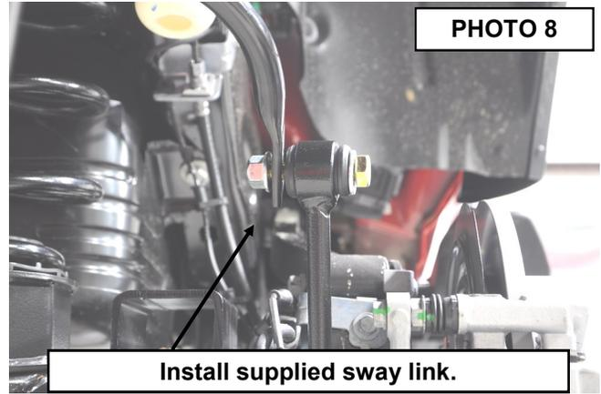
11. Using 18mm wrenches, tighten the upper sway link bolt. Torque to 75ft/lbs. **See Photo 9.**
