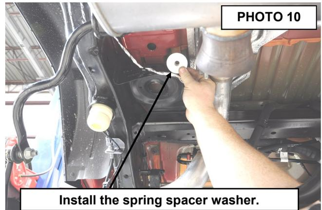
13. Install the supplied rear coil spacer, using the supplied 1/2" x 2.5" bolt (67730BAG3). Tighten using a 3/4" socket.
