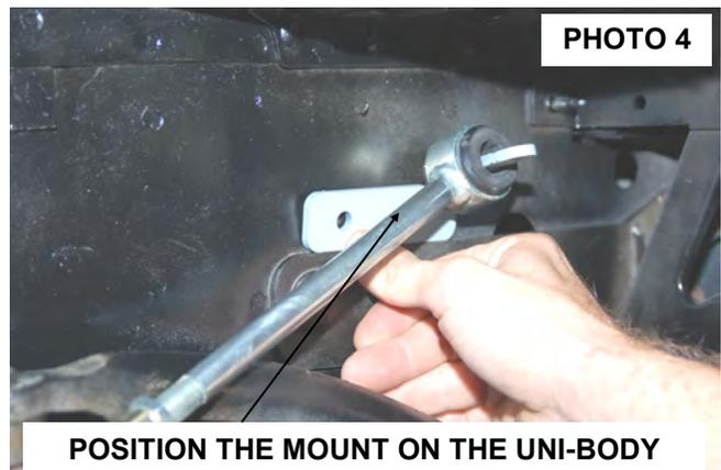
7. While holding the bracket in place, remove the sway bar link from the bracket. Mark and drill the holes using a 1/4" drill bit.
