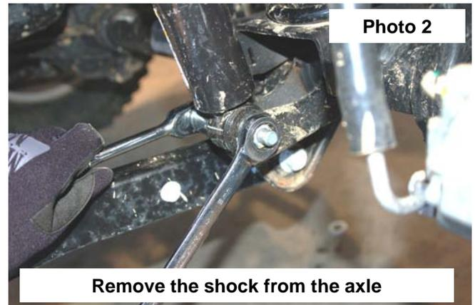
Remove the shock from the axle
