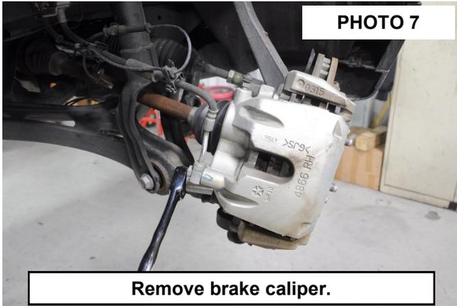
**Remove brake caliper.**
