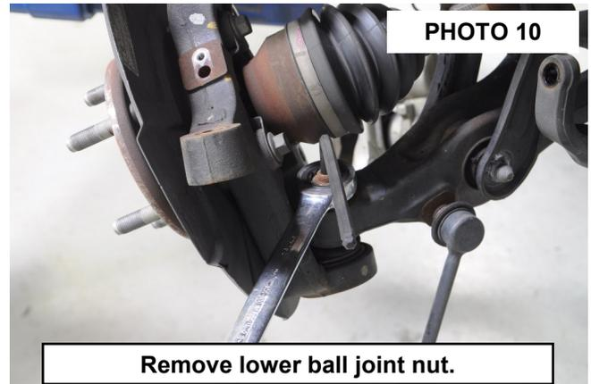
**Remove lower ball joint nut.**
