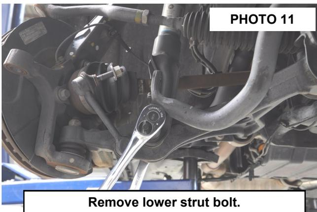
**Remove lower strut bolt.**
