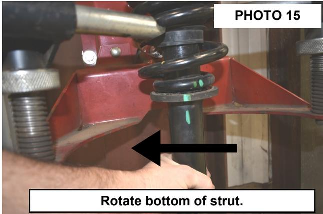
**Rotate bottom of strut.**
