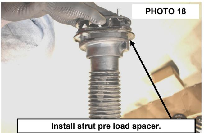
**Install strut pre load spacer.**
