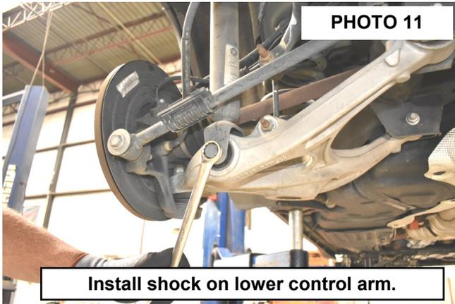
**Install shock on lower control arm.**
