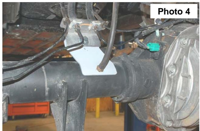
7. Using a 24mm socket, remove the stock u-bolts. Use the floor jack to lower the axle assembly to allow for lifted block installation. **See Photo 5. If equipped the factory block will not be reused.**
