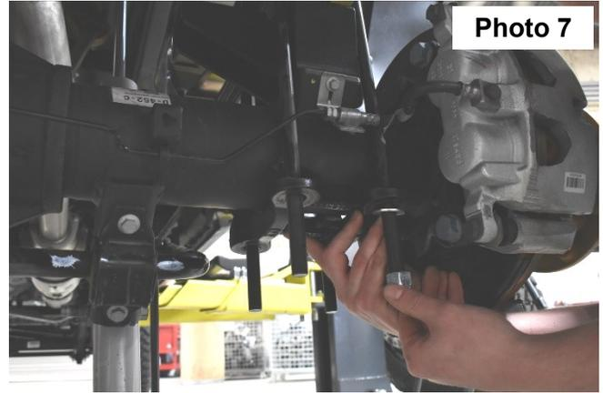
11. Locate shock part number 660805. Using an 18mm wrench, for the upper, and a 19mm and 15mm wrench for the lower. Install using factory hardware on upper and lower shock mount. Torque to 60 ft-lbs.
