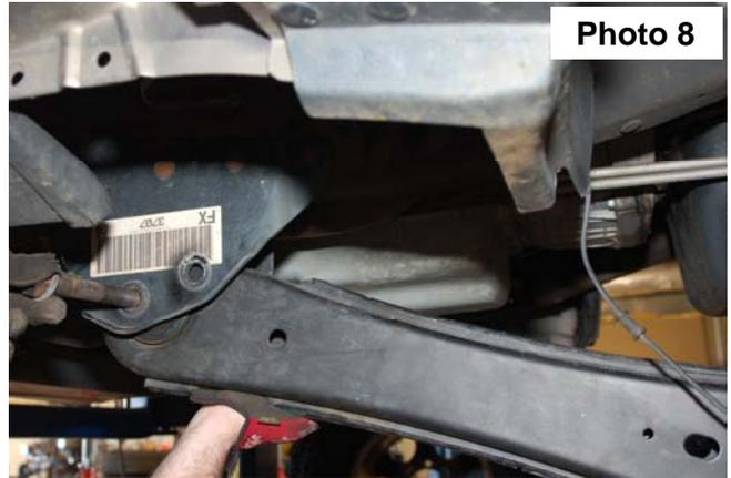
13. Insert the new supplied radius arm into the stock axle location. Use the stock bolt for the upper mount and the supplied 18mm x 130mm bolt, nut, and cam plates for the lower mount. **See Photo 9.**
