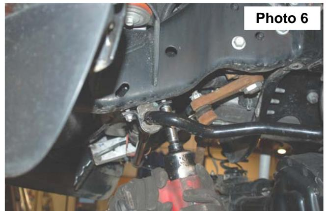
11. Support the radius arms with jack stands. Using a 24mm wrench, and socket remove the bolt holding the upper control arm to the axle. Retain stock hardware for reuse. **See Photo 7.**
