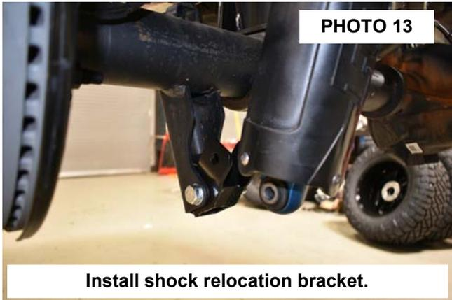
**Install shock relocation bracket.**
