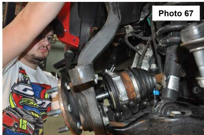
70. Using a floor jack, raise the lower control arm and connect the upper ball joint on the upper control arm to the spindle. Using a 21mm wrench, torque to manufacturer specs. If ball joint turns while tightening, use a 3/8" wrench to hold the ball joint.
