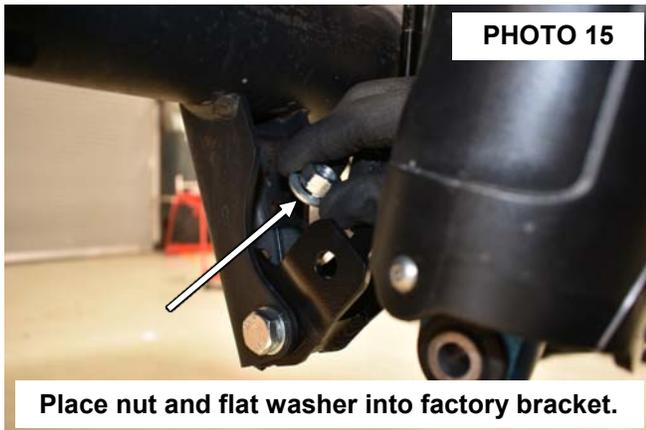
**Place nut and flat washer into factory bracket.**
