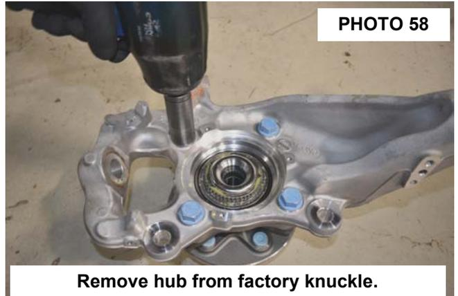
67. Remove the hub bearing assembly from the knuckle. **See Photo 59.**
