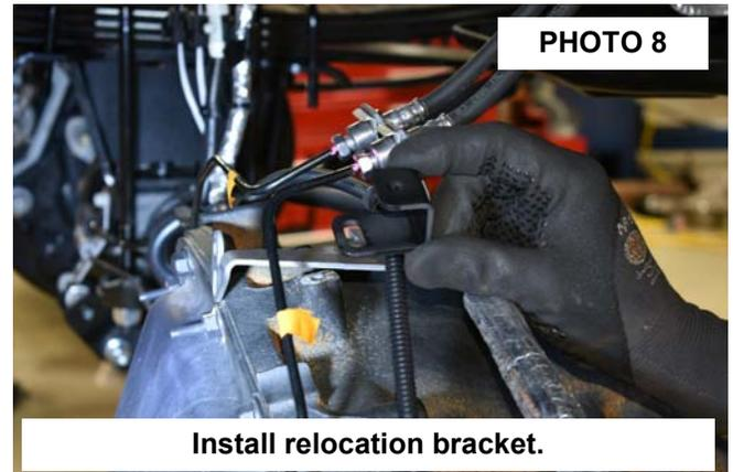
12. Attach the supplied relocation bracket to the differential using the factory hardware. Tighten using a 10mm wrench. **See Photo 9.**
