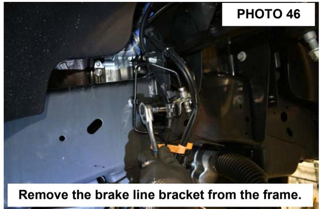
**Remove the brake line bracket from the frame.**
