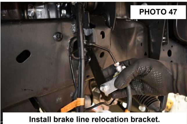
**Install brake line relocation bracket.**
