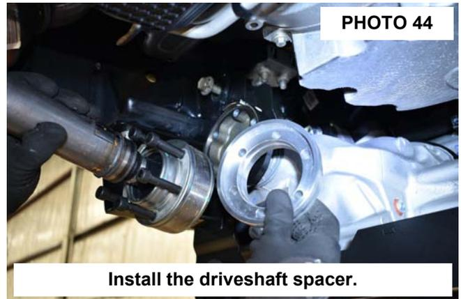
**Install the driveshaft spacer.**
