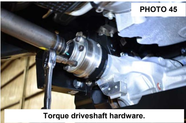
**Torque driveshaft hardware.**
