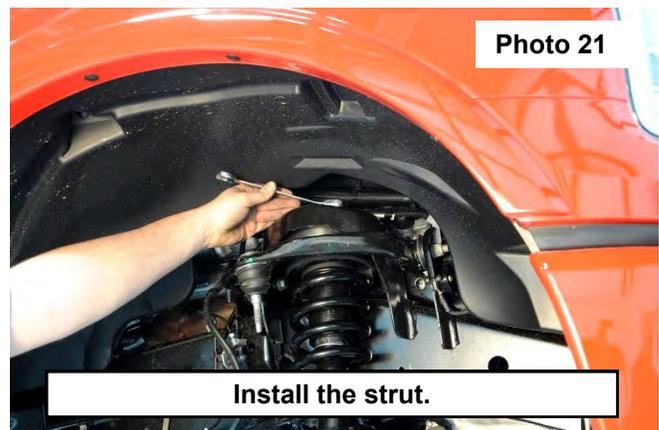
studs back into the barpin on the lower mount of the strut. It may be necessary to hit the top of the strut with a hammer to seat the splines before tightening the factory nuts with a 18mm. **See Photo 22.**
