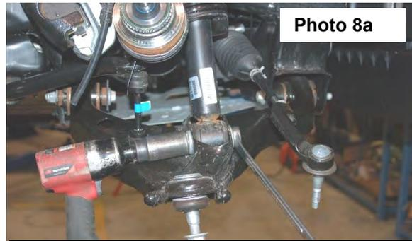
**Remove the lower strut bolt. 09-13 Models**
