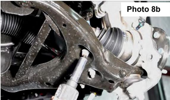
**Remove the lower strut bolts. 14-20 Models**
