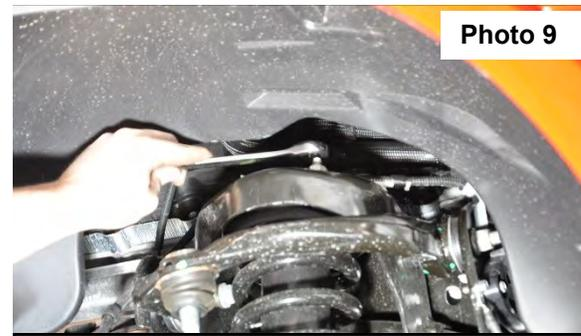
**Remove the upper strut nuts.**
