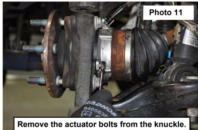
**Remove the actuator bolts from the knuckle.**
