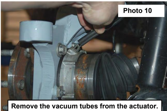
**Remove the vacuum tubes from the actuator.**
