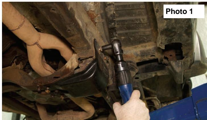
Remove the Torsion bar protector plate.
