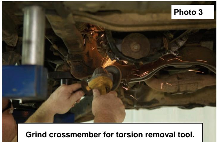
5. **WARNING** Use extreme caution when loading and unloading the torsion bars; there is a tremendous amount of energy stored in them. Keep your hands and body clear of the adjuster arm assembly and the puller tool in case anything slips or breaks.
