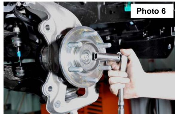
9. Using a 21mm wrench and a 1 1/16+socket loosen the lower control arm bolts. Do not remove the bolts just loosen them so you can later swing the lower control arm down.
