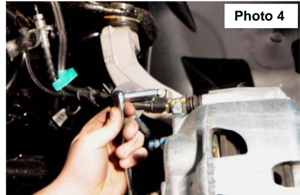
6. Next remove the caliper bolts with a 18mm socket as shown in **Photo 5** and the dust shield bolts with a 8mm socket. Remove the ABS wire from the knuckle with a 5mm allen wrench.
