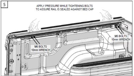
5. Once the mounting rails are in place, apply pressure while tightening the bolts to assure rails are sealed against the bed cap. (The use of a ratchet, 10MM socket or wrench for the M-6 bolts is recommended). The assistance of another person may be needed for this step to get the proper seal.
