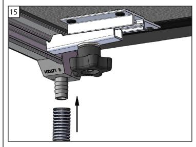
15. Attach the drain tubes to the fittings at the front of the bed rail and position the tubes to divert water out of the truck bed. This can be done by placing the tube behind a bed liner, through an existing hole in the bed, or by drilling a 5/8" hole in the bulkhead.
