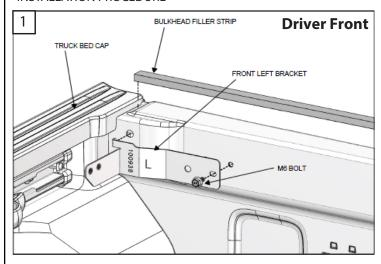
CUT AND REMOVE PORTION OF BED CAP TO REVEAL THREADED HOLES
