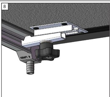
7 & 8. Assemble the four retainer clamps, slide each of them into the track on the underside of the tonneau, slide into position, but do not tighten at this time.
