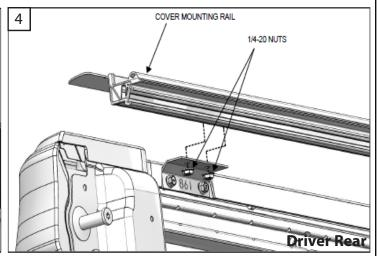
4. Install the rear portion of each mounting rail, (as shown in Drawing 4) Locate the 2 studs on the bottom side of the mouting rail and place the studs through the 2 holes in the rear bracket. Use 2 (1/4-20) nuts, thread on to the studs and tighten, using a 7/16" socket. Repeat process for opposite side.
