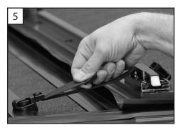
3, 4 & 5. Release the strap from the stowed position by squeezing the tabs. Attach the buckle at the bulkhead, pull the strap to take up the slack and secure the cover. Repeat this for the opposite side.
