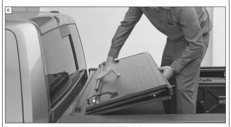
6. Set the tonneau onto the mounting rails, the buckles should be to the front.
