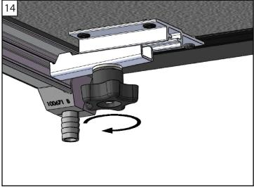
13 & 14. Once in the open position double check the clamp engagement to the side rail and tighten. Test the cover again for proper operation, adjust as needed, then tighten the star knobs.
