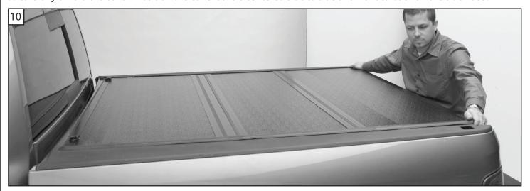
10. Test the rear latching assembly for smooth operation as this is the best indicator of the cover being posi-tioned correctly. Be sure the latches on both sides are engaging with the cover mounting rail.
