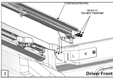
3. Locate the Driver side mounting rail. Using 2 M-6 flange head mounting bolts, install the driver side mounting rail to the driver side front bracket (as shown in Drawing 3). Do not tighten, leave slightly loose until rear mounting bolts are installed. Repeat process for passenger side.
