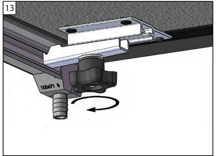
12 & 13. Once in the open position double check the clamp engagement to the side rail and tighten. Test the cover again for proper operation, adjust as needed, then tighten the star knobs.
