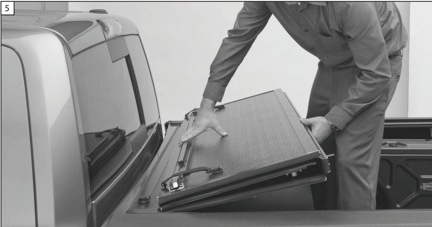
5. Set the tonneau onto the mounting rails, the buckles should be to the front.
