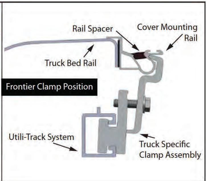
3. Using three (3) clamps per side attach the rail to the bed, position the clamps adjacent to each of the black rail spacers. (Tip: Mount the center clamp first but do not tighten completely. This will give you the ability to adjust the rail as the outer clamps are attached)
