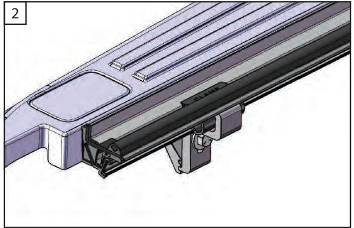
1. Attach both left and right side rails to the truck bed. The end of the mounting rail with the drain tube fitting will go towards the cab of the truck, position flush to bulkhead.
