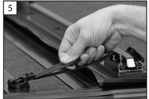
3, 4 & 5. Release the strap from the stowed position by squeezing the tabs. Attach the buckle at the bulk-head, pull the strap to take up the slack and secure the cover. Repeat this for the opposite side.
