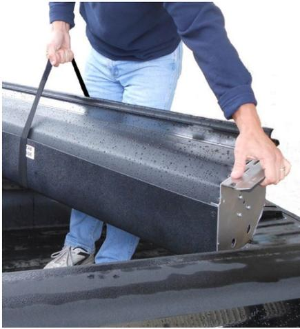
Place the Canister in the truck bed just behind the cab and center it from side to side. Ensuring that the canister is centered in the bed will help assemble the rails to the canister in the next step.
