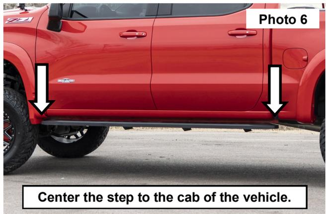
7. Adjust the inside of the step plate within a 1/4" away from the cab of the vehicle. **See Photo 7.**
