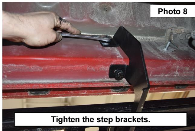
9. Tighten the hardware using a 10mm wrench on each of the (4) mounting brackets. **See Photo 9.**
