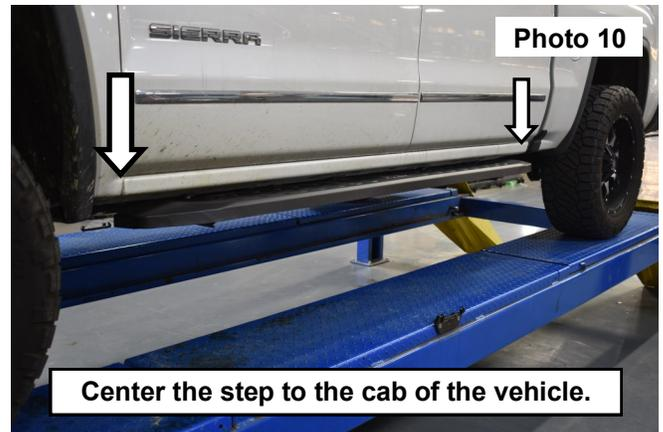
10. Adjust the inside of the step plate within a 1/4" away from the cab of the vehicle. **See Photo 11.**
