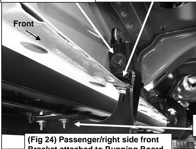
(Fig 24) Passenger/right side front Bracket attached to Running Board
