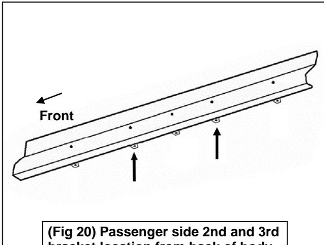
(Fig 20) Passenger side 2nd and 3rd bracket location from back of body
