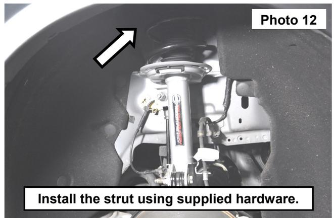
14. Secure the strut using the supplied hardware and tighten using a 13mm socket **See Photo 13.**
