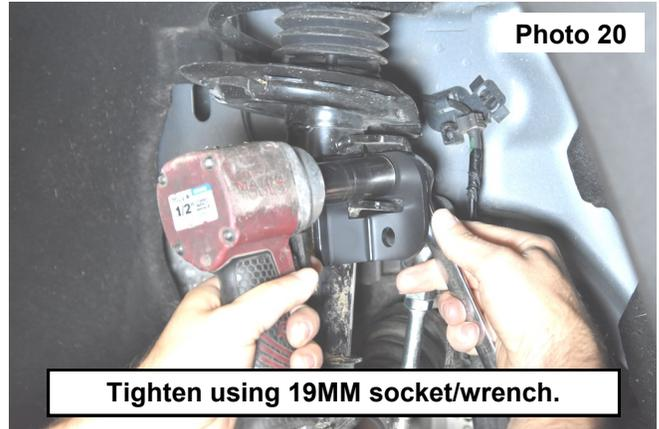
20. Install the upper swaybar link using a 19MM socket/wrench. **See Photo 21.**
