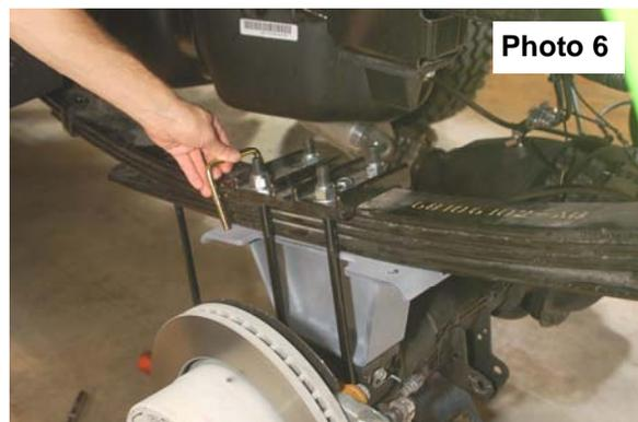
11. Assemble the new shock absorbers part # 658728 with bushings/sleeves and install on the vehicle.
