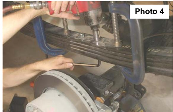
9. Remove C clamps and install supplied anti-wrap block and u-bolts. Tighten using a 13/16" socket. Torque to 90 ft-lbs. **Larger end of the block will go toward the rear of the truck. See Photo 5.**
