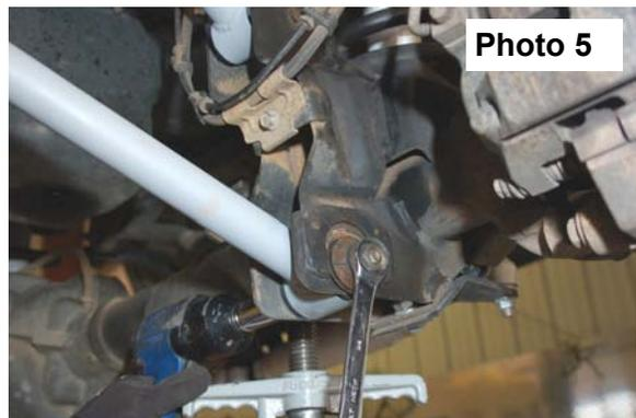
9. Install the new Rough Country lower suspension arms in place of the stock lower suspension arms as shown in **Photo 5**. Slight prying of the mounts may be necessary for arm installation. Install the original rear suspension arm bolt and slightly tighten the nut. Install the original front suspension arm bolt and slightly tighten the nut. Refer to the reference mark on the cam bolt and the axle when installing the cam bolt.
