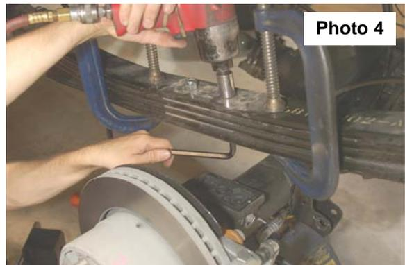
9. Remove C clamps and install supplied anti-wrap block and u-bolts. Tighten using a 13/16" socket. Torque to 90 ft-lbs. **Larger end of the block will go toward the rear of the truck. See Photo 5.**
