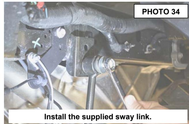
41. Install the sway link on the sway bar using the supplied 12mm x 65mm bolt, large washer, and flange lock nut (33430BAG6). Torque to 55ft/lbs using an 18mm socket and wrench. **See Photo 35.**
