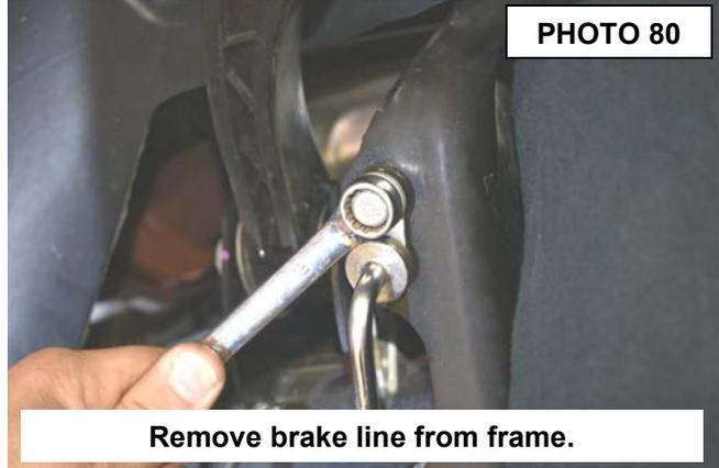
**Remove brake line from frame.**
