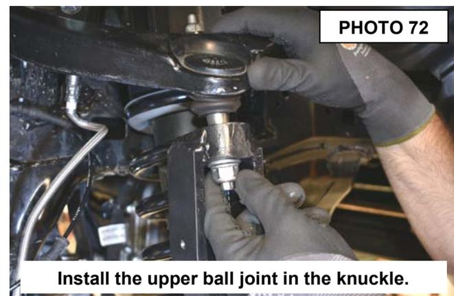
81. Tighten the upper ball joint using a 21mm wrench.. **See Photo 73.**
