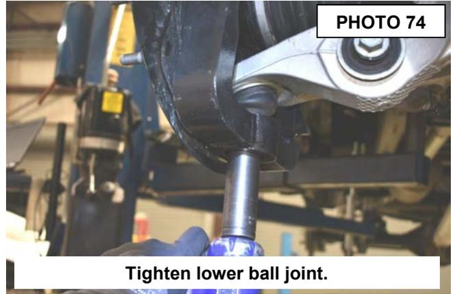
**Tighten lower ball joint.**
