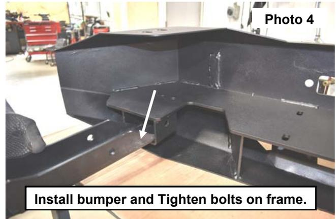
4. Slide the EXO bumper back, to line up the holes in the brackets, use the supplied 12mm x 120mm bolts, washers and lock nuts. Do not fully tighten at this time. **See Photo 5.**
