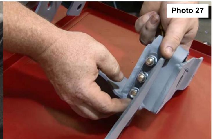
32. Install upper control arm drops onto truck using supplied 9/16" x 4" bolts and nuts using four cam lock washer per side with one cam lock washer with a tail on the back side for the ABS wire. **See Photo 29.**
