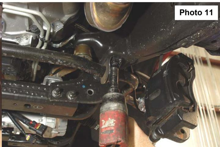
16. Remove the lower control arm using a 18mm wrench and a 24mm socket. **See Photo 12.**
