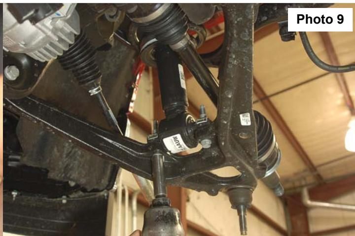
14. Remove CV axle bolts using a 15mm socket. **See Photo 10**.
