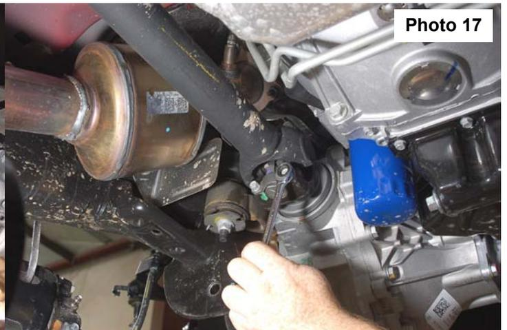
22. Support diff. Using a 18mm socket and 21mm socket remove the bolts from diff. lower diff from truck. **See Photo 18.**
