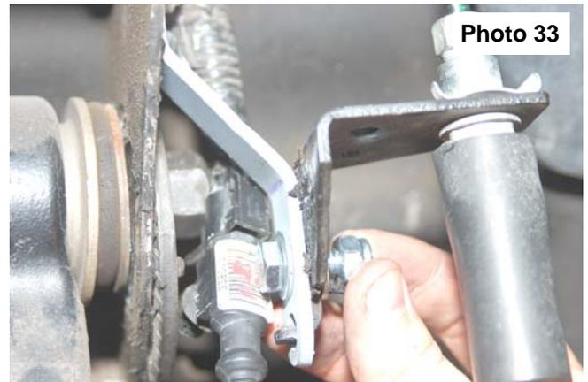
52. Remove the brake line clip from the brake line using a flat head screw driver as shown in **Photo 34** and trim as shown in **Photo 35**. Reinstall the modified bracket on the stock control arm with the stock hardware.
