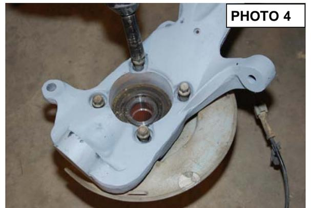
15. Using a 9/16+wrench remove the sway bar link.
