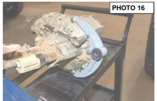
30. Install the differential as shown with stock hardware in the rear lower hole and using the supplied 1/2-x 1 1/2+hardware on the passenger side in 1297BAG1 as shown in **Photo 17**.
