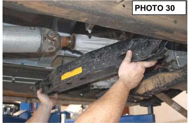
45. To ease installation, install the factory torsion bars in the lower control arms and slide forward slightly. Locate new torsion bar drop bracket over the factory rivets on the side of the frame rail as shown in **Photo 31** and clamp in place. Using the bracket as a guide, drill holes using a 17/32+drill bit.
