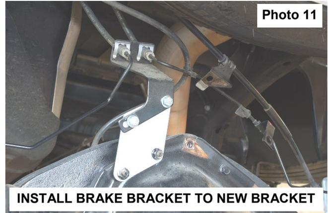
16. Install the supplied brackets on the differential with the stock hardware. **See Photo 12**. Tighten using a 13mm socket / wrench. Reinstall the stock brake line brackets on the new brackets using the supplied 5/16" x 3/4" bolts, flat washers and lock nuts from 1253Bag4. Tighten using a 1/2" socket / wrench.
