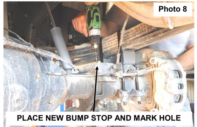
13. Install the supplied bump stop and secure with the supplied 3/8" self tapping bolt from 1260bag2. Tighten with a 9/16" socket. **See Photo 9.**
