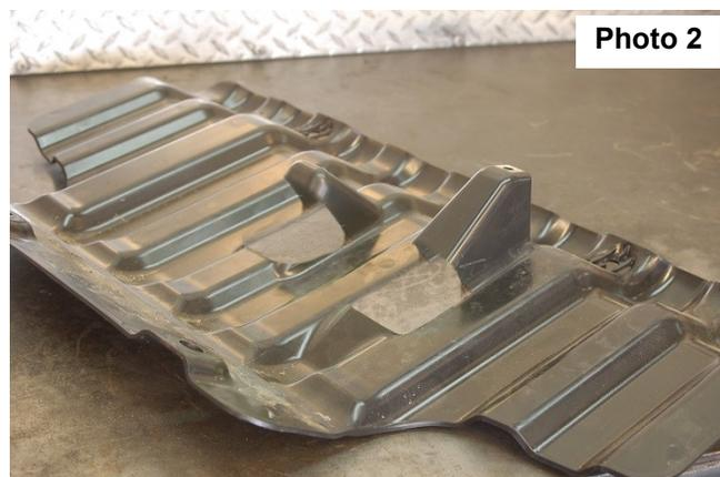
4. After this area is cut bolt the skid plate back in factory location use the four factory bolts. Tighten with a 15mm socket.
