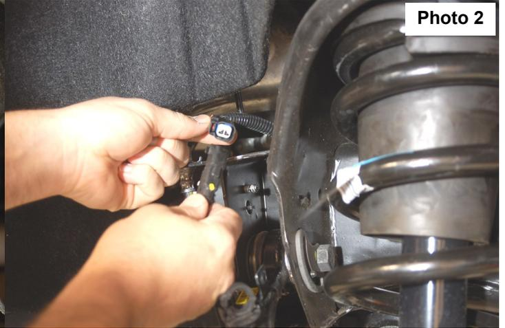
5. Remove the sensor wire from the plastic clip. Remove the brake line bracket from the control arm using a 10mm wrench. **See Photo 3.** Next remove the bracket line bracket from the control arm pocket with a 13mm wrench.
