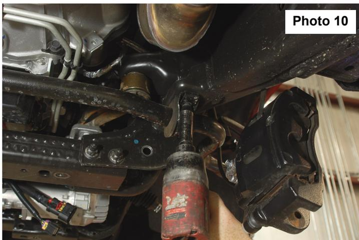
14. Remove the lower control arm using a 18mm wrench and a 24mm socket. **See Photo 11.**
