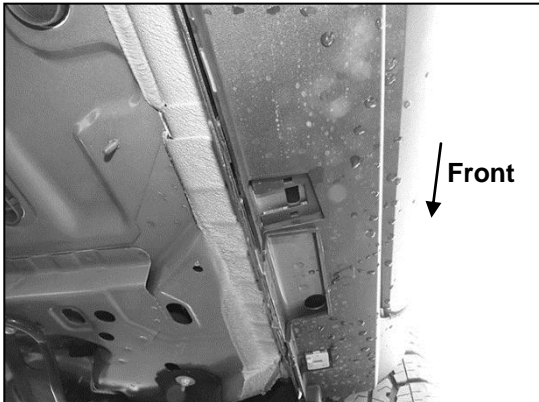
(Fig 3) Plastic clip removed from the front location trim (Passenger side shown)
