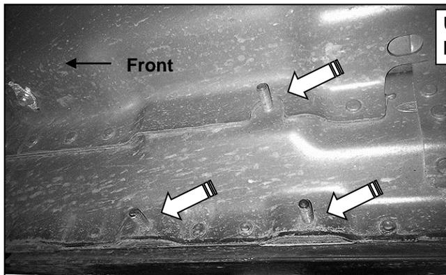
Use a wire brush to remove paint from threads
