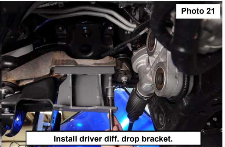
25. Install the diff using the supplied 12mm bolts and flange nuts on the driver side and 12mm bolts with stock nuts on the passenger side. Do not tighten at this time.
