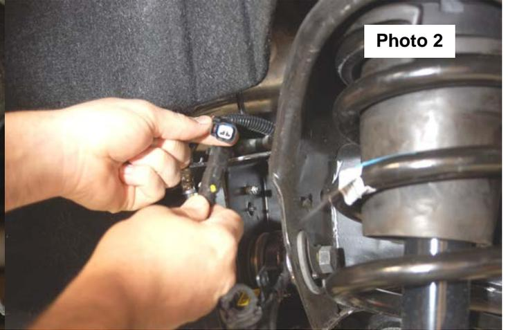
5. Remove the sensor wire from the plastic clip. Remove the brake line bracket from the control arm using a 10mm wrench. **See Photo 3.** Next remove the bracket line bracket from the control arm pocket with a 13mm wrench. Using a 3/8" wrench, remove the Magneride linkage from the brackets.
