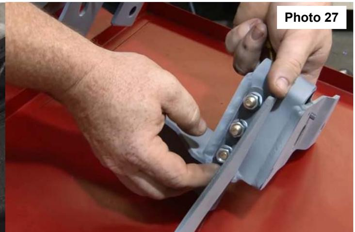
32. Install upper control arm drops onto truck using supplied 9/16" x 4" bolts and nuts using four cam lock washer per side with one cam lock washer with a tail on the back side for the ABS wire. **See Photo 29.**
