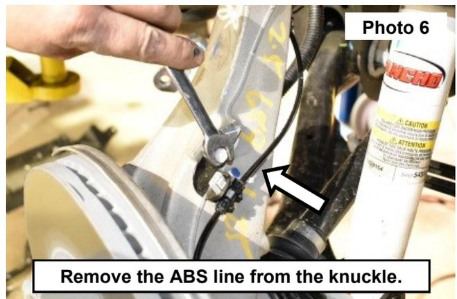
9. Remove the ABS sensor from the knuckle using a 10mm wrench. Retain hardware for reuse. **See Photo 7.**
