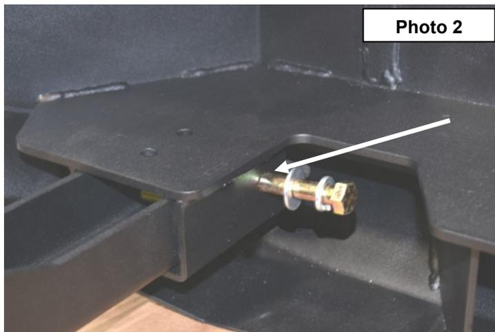
3. Install the supplied 1/2" x 3 1/2" bolts in the frame bracket as shown with the flat washers and lock nuts. **See Photo 3.**
