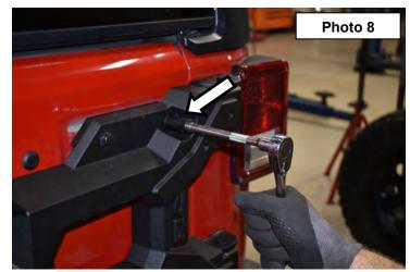
8. **NOTE:** The height of this bracket can be adjusted when fitting the wheel and tire. Install the carrier bracket on to the mounting plate using (6) of the supplied 10mm x 30mm Button head bolts, flat washers and (6) 10mm flange lock nuts. Tighten the hardware using a 6mm allen and a 14mm wrench. **See Photo 9 and 10**.
