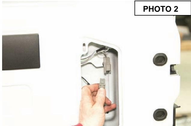
3. Close tailgate, remove rubber grommet holding the 3rd brake light wires. **See Photo 3**
