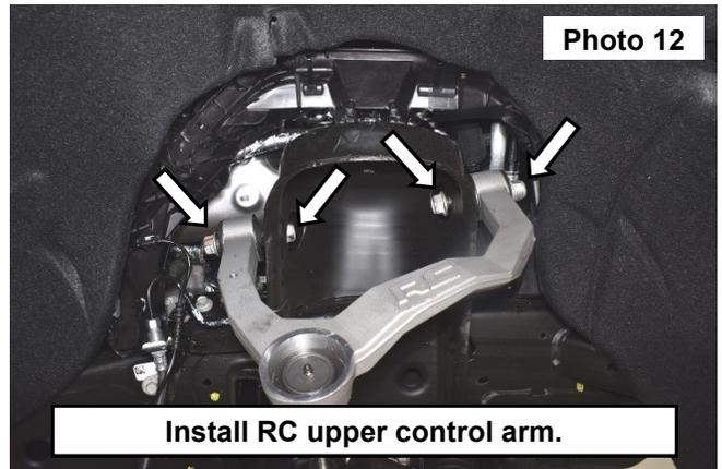
14. Reassemble suspension in reverse order of tear down.
