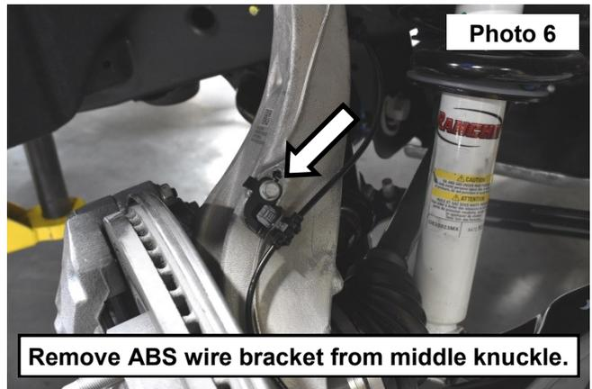
8. Remove the ABS wire from the lower knuckle using a 10mm socket/wrench. **See Photo 7.**
