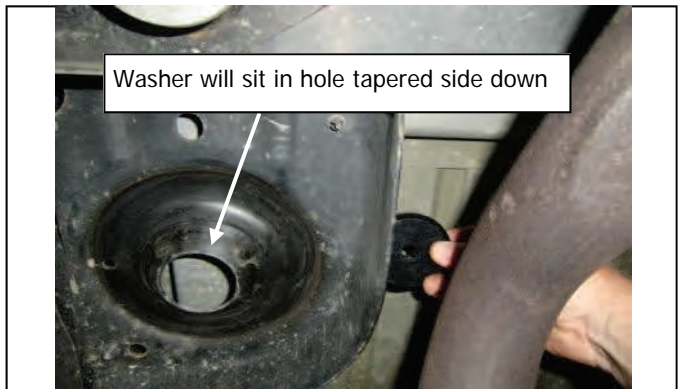
Place threaded washer above upper spring mount as shown
