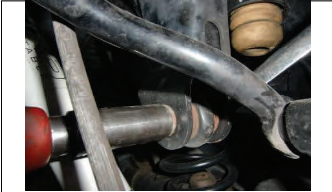
Slightly lift rear axle and remove upper trac bar bolt.
