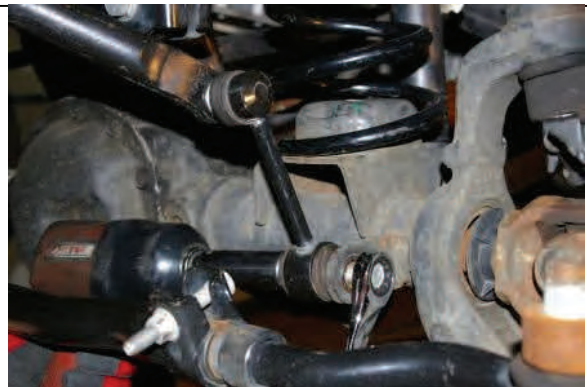
Disconnect dr./pass. lower front swaybar endlinks
