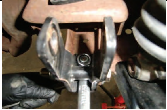
Install front lower shock extensions and torque to spec
