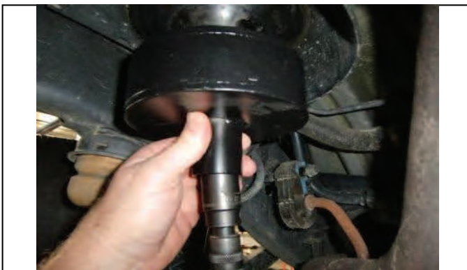
Bolt spacer into position by hand using short socket/ext
