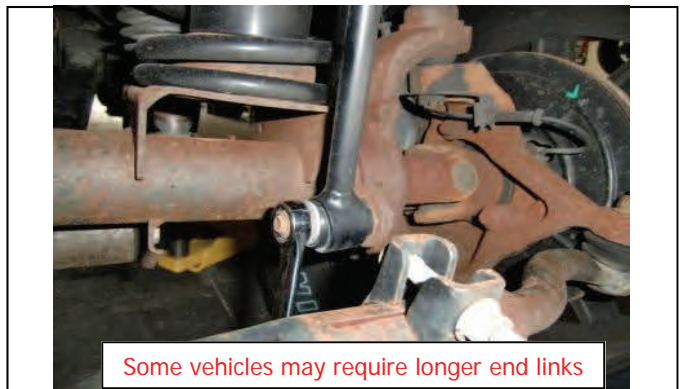
Reattach front sway bar end links .
