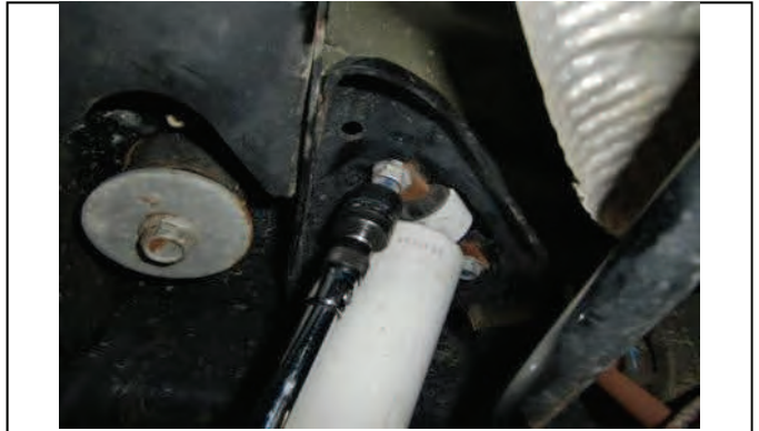
Next, remove rear upper shock bolts.
