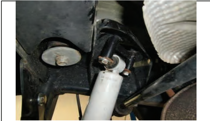
Install upper shock extensions with provided hardware.
