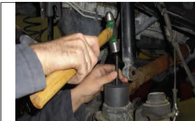
Center, mark and drill 11/32 hole for self tapping bolt.
