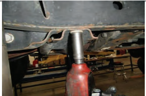
Reinstall front transfer case skid plate bolts.
