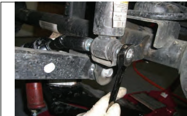
Disconnect and remove front lower shock hardware.
