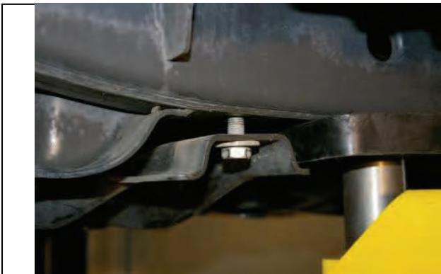
Remove (2) front transfer case skid plate bolts.
