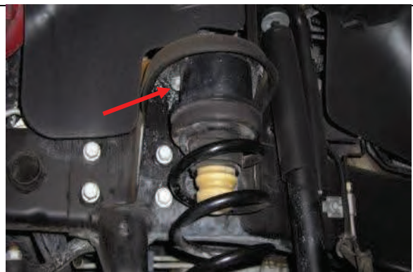
Bolt-in spacers, install OE isolator, then bumpstops & springs
