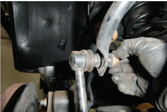
Disconnect rear sway bar end links
