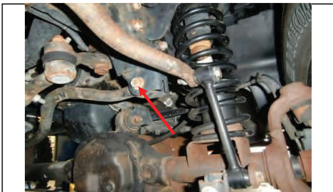
Reconnect front upper trac bar with OE hardware and torque.
