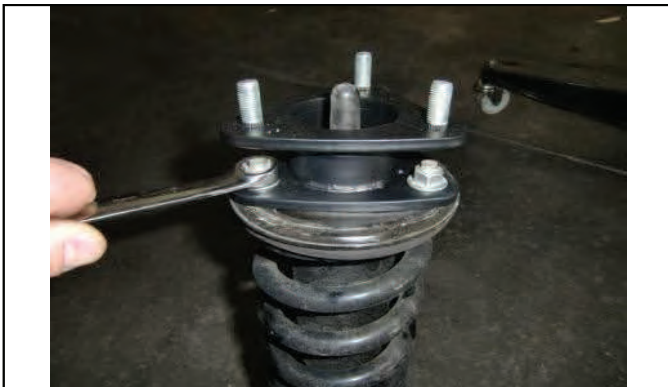
Attach strut extension with OE hardware
