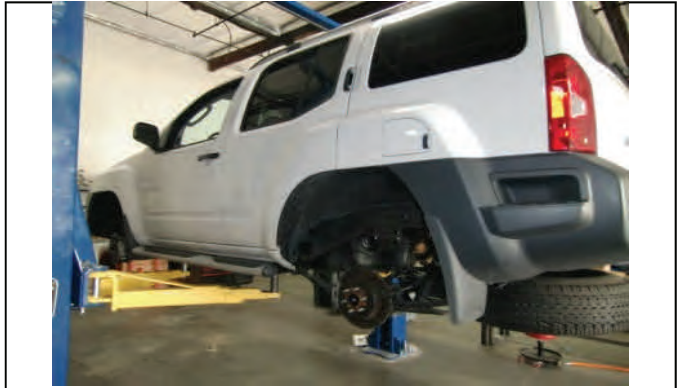
Raise and support vehicle by frame
