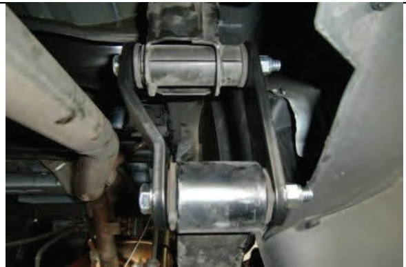
Tighten new hardware
