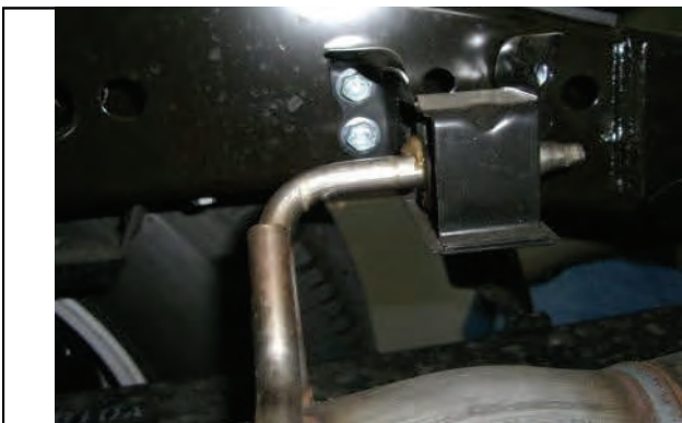
Unbolt rearmost exhaust hanger on frame
