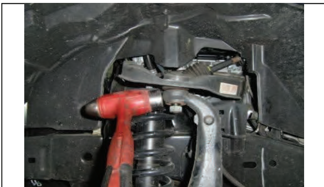
Strike spindle to break loose connection
