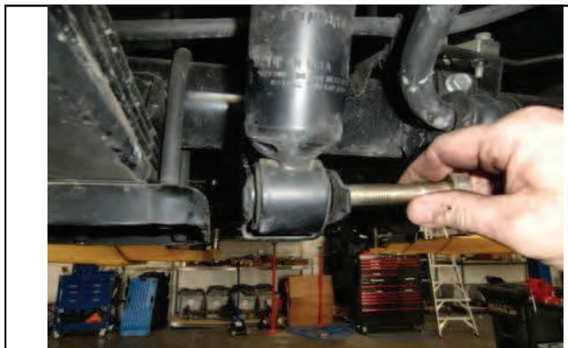
Remove lower shock mounting hardware
