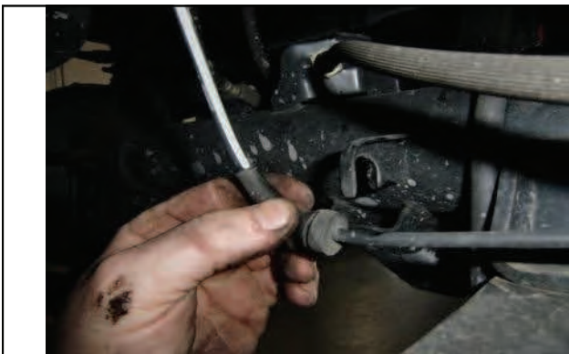
Remove ABS lines from attachments on axle
