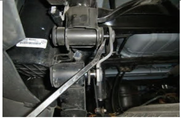
Pry out the inner shackle mounting bracket
