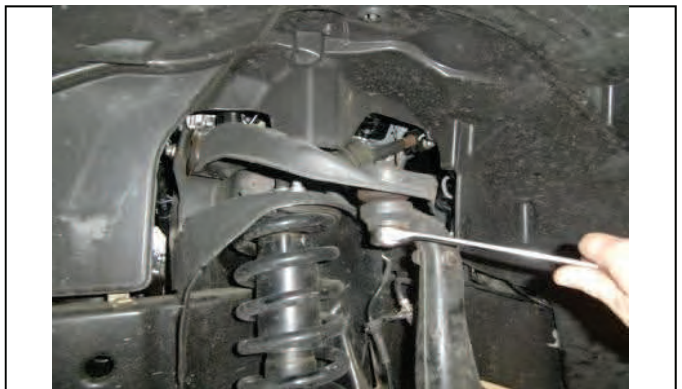
Loosen upper ball joint nut, do not remove
