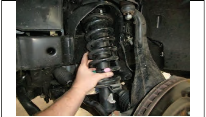
Remove strut assembly from vehicle
