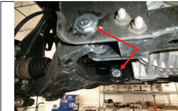
Orient cams in the upright/neutral position and tighten
