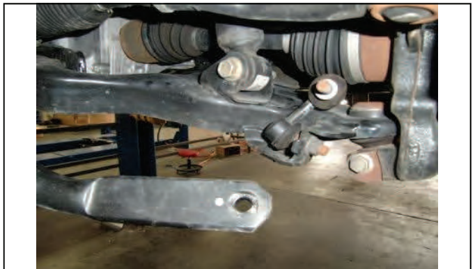
Disconnect sway bar end links
