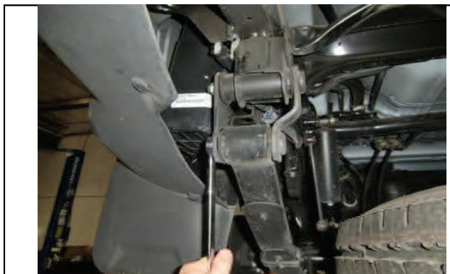
Unbolt the upper/lower shackle hardware
