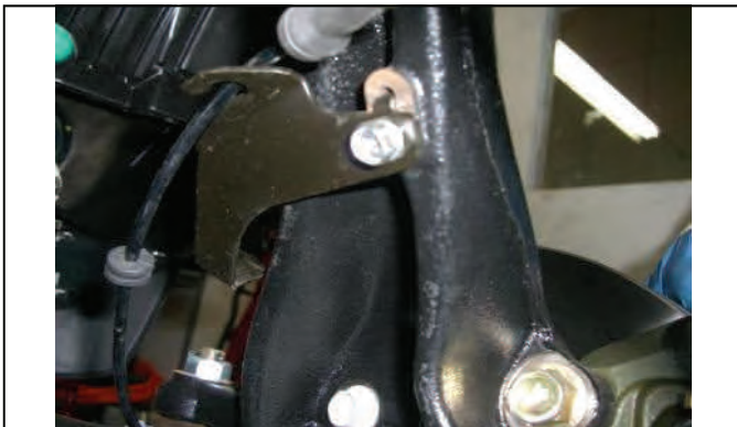
Disconnect ABS line bracket behind spindle
