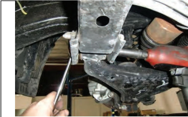
Loosen the lower control arm mounting hardware
