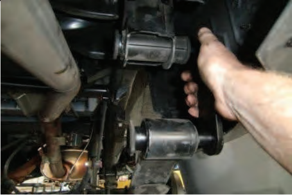
Lower axle and install new shackle bracket
