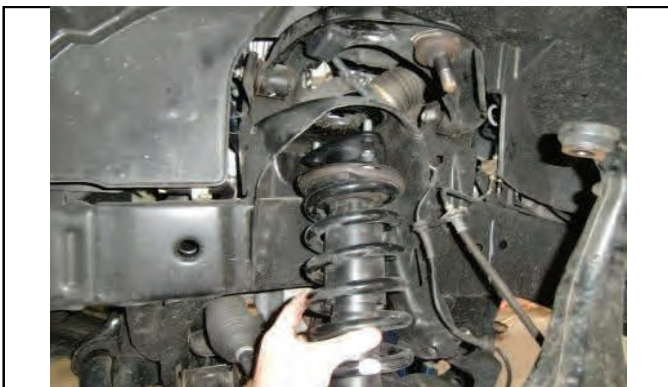
Reinstall strut assembly into vehicle w/ new upper hardware
