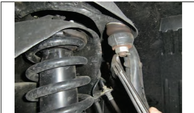
Remove cotter pin and upper ball joint
