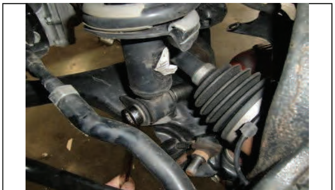
Remove lower shock mounting hardware
