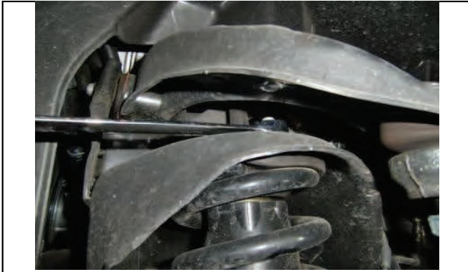
Remove upper strut mounting hardware
