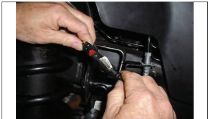
Reconnect ABS plug near frame
