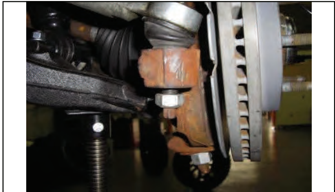
Reconnect outer tie rod end and tighten
