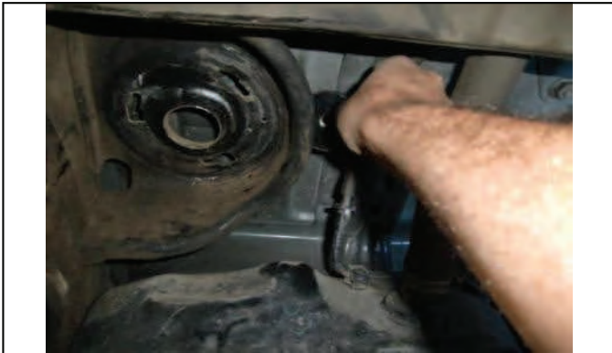
Place Upper coil spacer nut plate above coil housing
