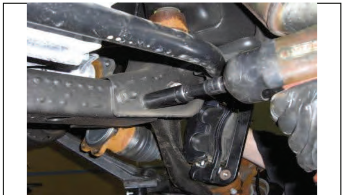
Unbolt rear cross member (4) bolts and remove
