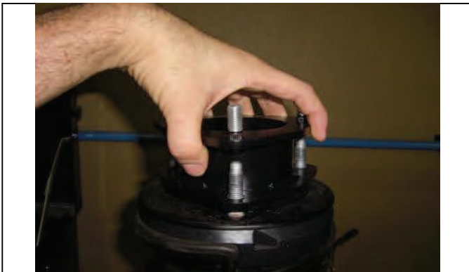
Place new strut extension spacer onto strut
