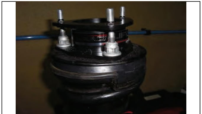
Attach and tighten with OE hardware
