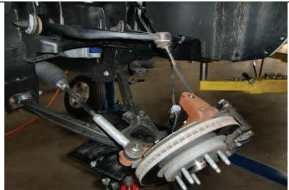
Carefully separate ball joint from spindle
