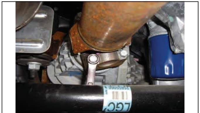
Disconnect U-joint straps at differential yoke, slide back
