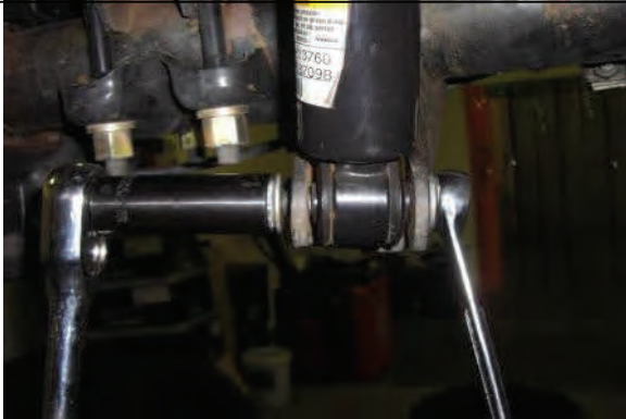
Disconnect and remove rear shocks from vehicle
