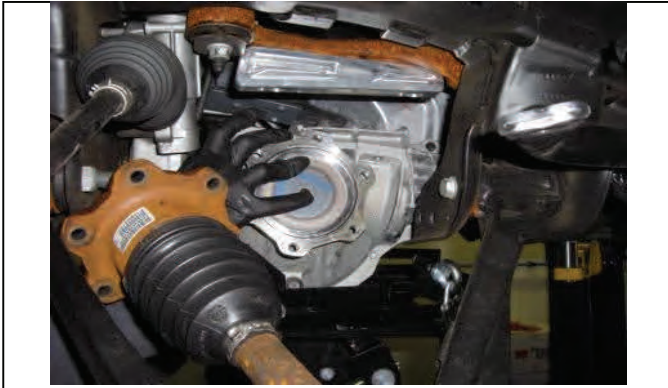
Raise and position diff back into vehicle check clearance
