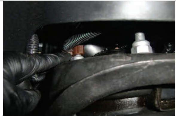
Remove clips from top of upper strut mounting nuts
