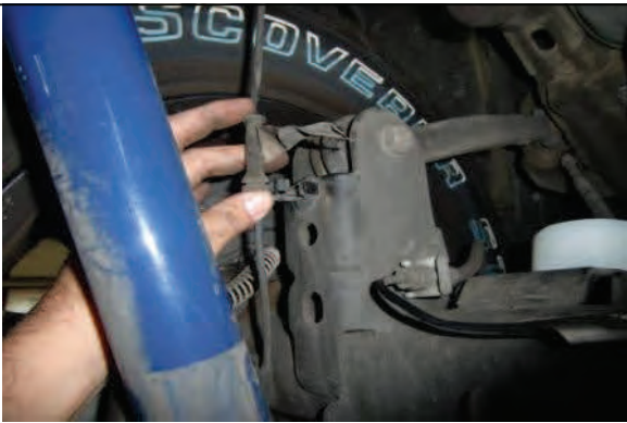
Disconnect ABS/TC line at the axle to avoid damage.
