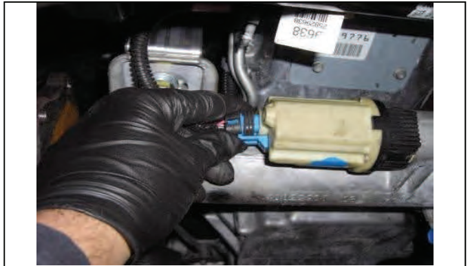
Reconnect differential solenoid
