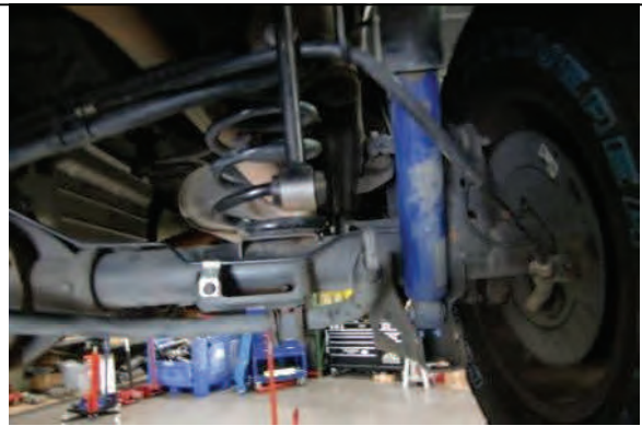
Disconnect and remove sway bar end links and shocks
