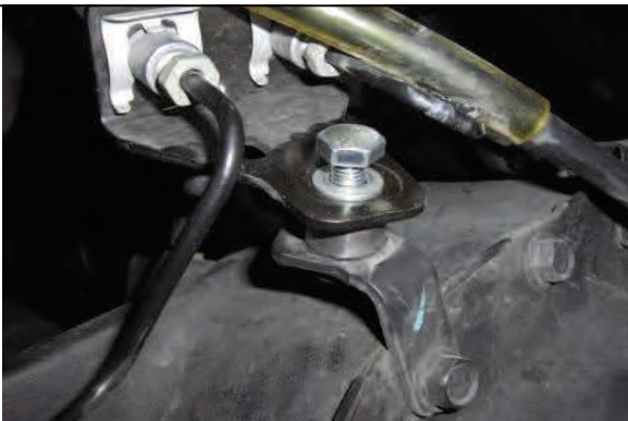
At the differential, install spacer and hardware as shown
