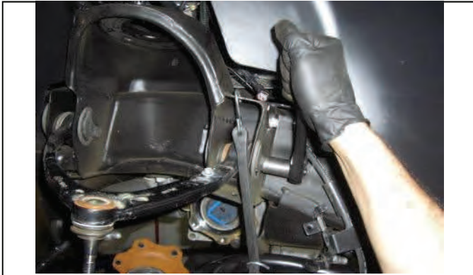
Unbolt upper control arms hardware, note cam location
