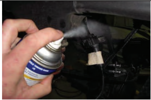
Lube ABS wire and slide rubber mount up to gain more slack
