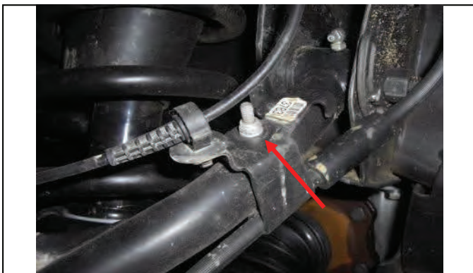
Attach ABS/brake line bracket to upper control arm
