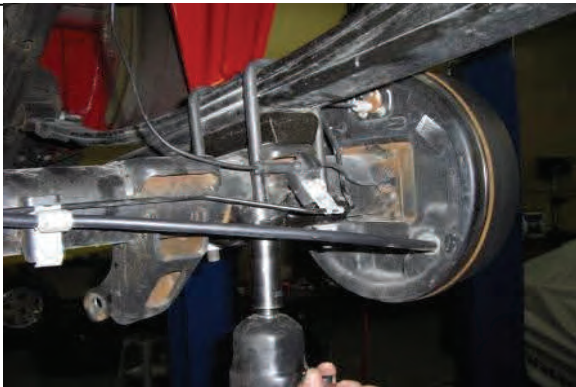
With axle supported remove u-bolts from axle
