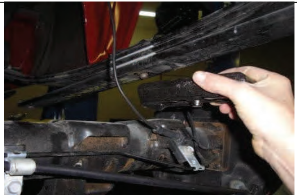
Carefully lower axle and remove factory block, do not reuse
