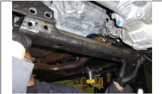
Reinstall rear cross member as original
