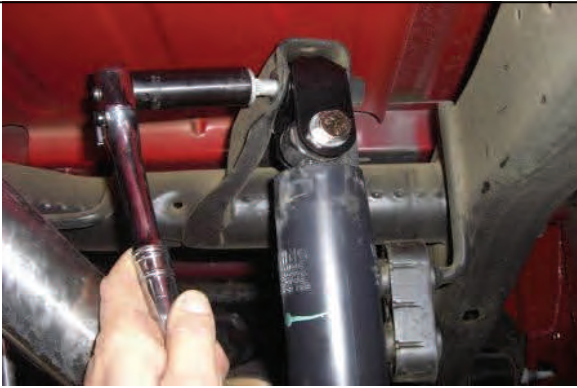
Reinstall shock with extension attached and tighten
