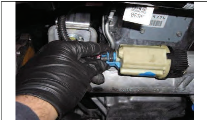
Unplug differential solenoid
