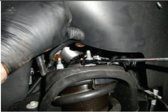
Remove upper mounting nuts
