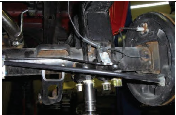
Raise axle align and attach new u-bolts and hardware
