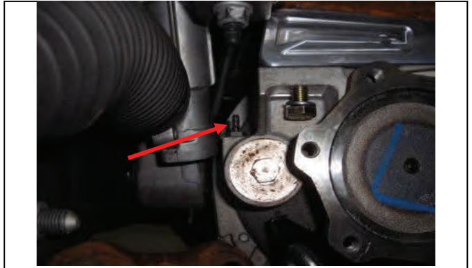
Attach with new hardware and reconnect differential vent line
