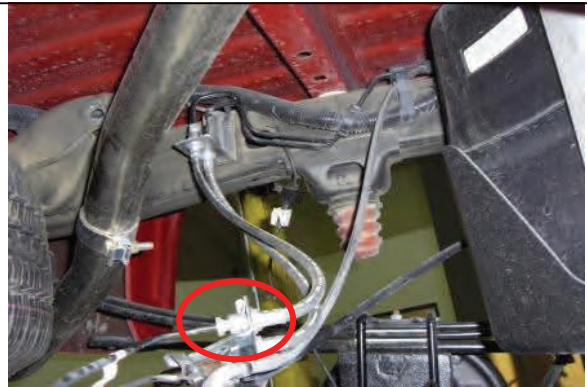
Differential brake line bracket made require bending up
