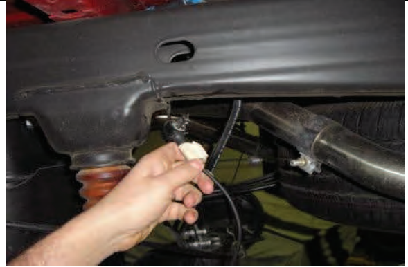
Unclips ABS/traction control lines at the frame
