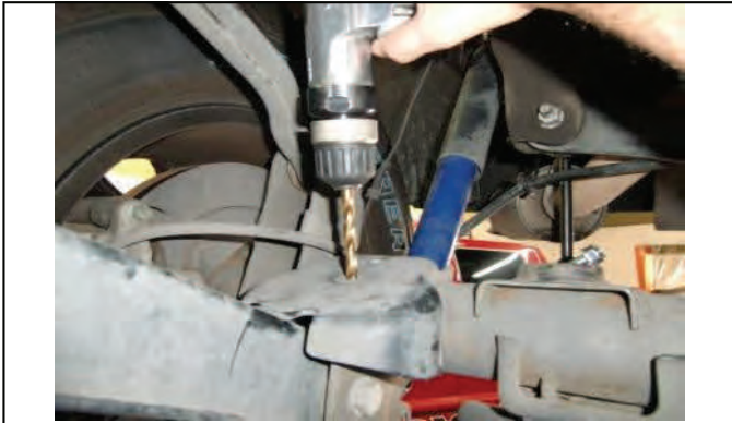
Mark center of bump stop pad and drill 11/32 hole
