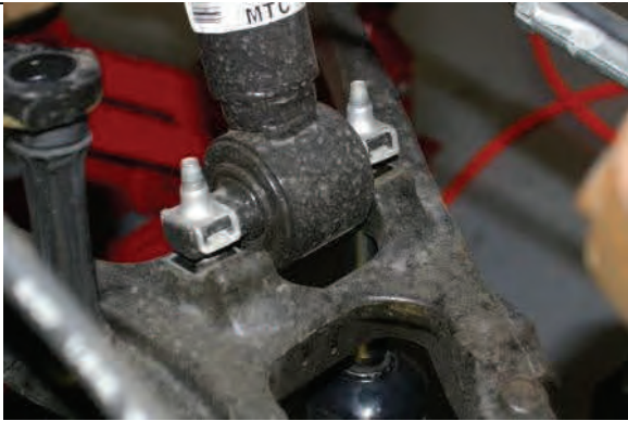
Remove lower strut mounting hardware, remove nut clips
