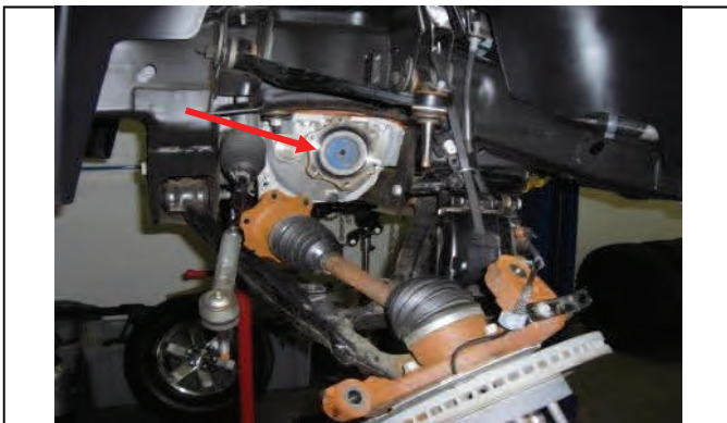
Unbolt CV axles (6) bolts at the differential
