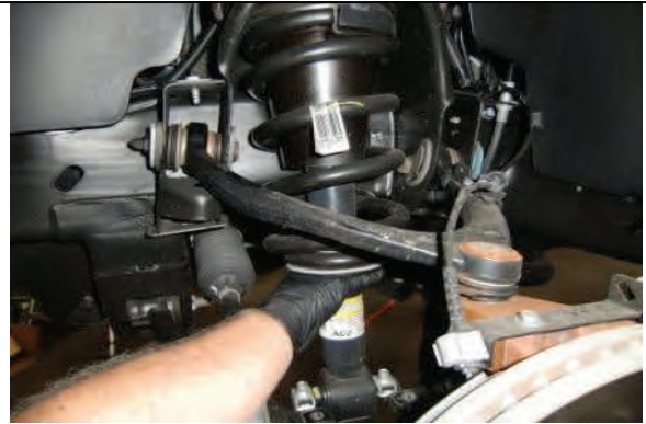
Remove strut assembly from vehicle.
